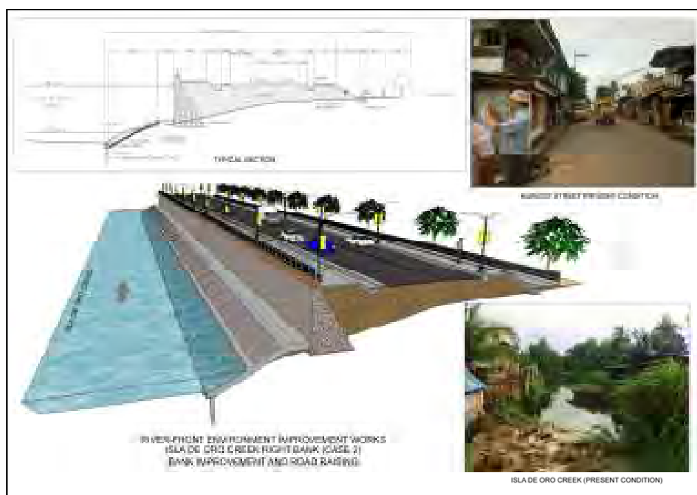
Figure 2.3.11 Typical Section of Concrete Wall & Boulevard (2 Lanes Road)
