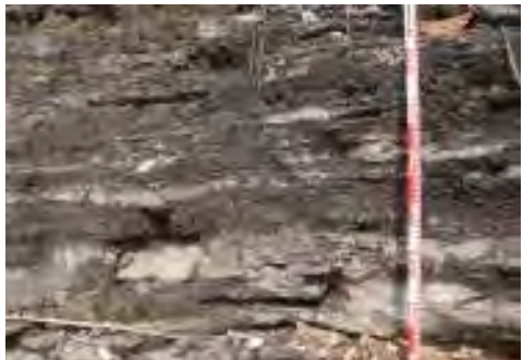
Siliceous Sandstone (near airport) (Alternate of Limestone and Sandstone) Slope failures are observed in several places; Weak resistance to erosion
