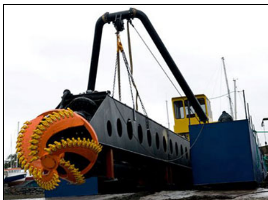
Figure 56: The 'business-end' of a cutter-suction dredge – the 'cutter-head'. Any marine life that comes in contact with it when operating will be destroyed/severely damaged (Source: dredgebroker.com)
