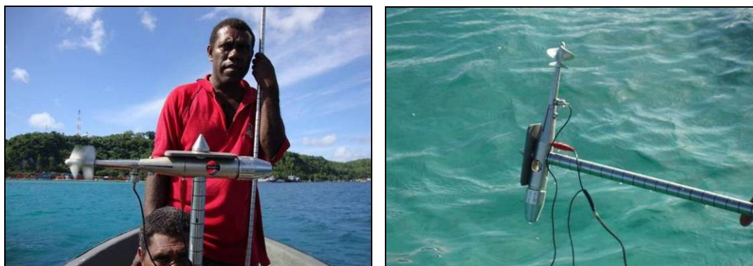
Figure 3: Close up of the OTT current probe propeller unit
