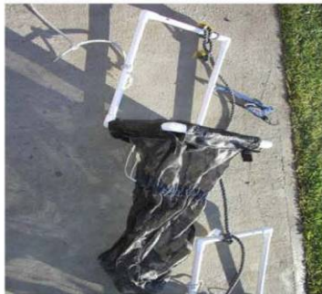
Figure 1: The quadrats (40 cm x 25 cm) used to sample fouling assemblages (left) were fastened to the wharf piles using bungy cords. Samples scraped from the piles (right) were captured in a 1 mm mesh sample bag suspended below the quadrat.
