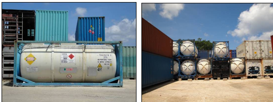
Figure 61: Tanktainers of avgas and diesel, and containers with contents of paints, solvents, aerosols and other hazardous materials may be handled at the new Star Terminal. These will need to be managed in accordance with the IMDG Code (Source: Raaymakers).
