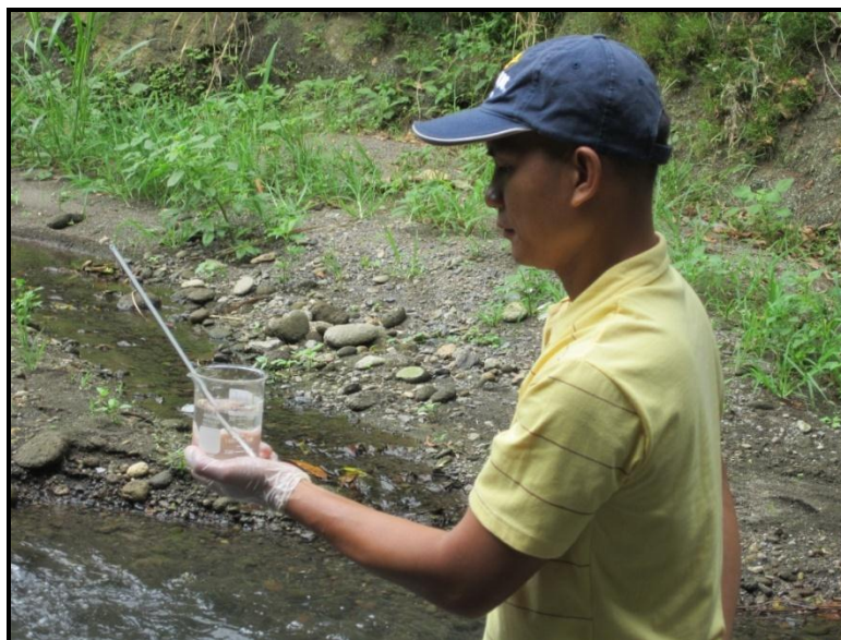
Plate No. 17 Temperature measurement of sample collected from Malindig River, Sta. 3 using a laboratory thermometer.
