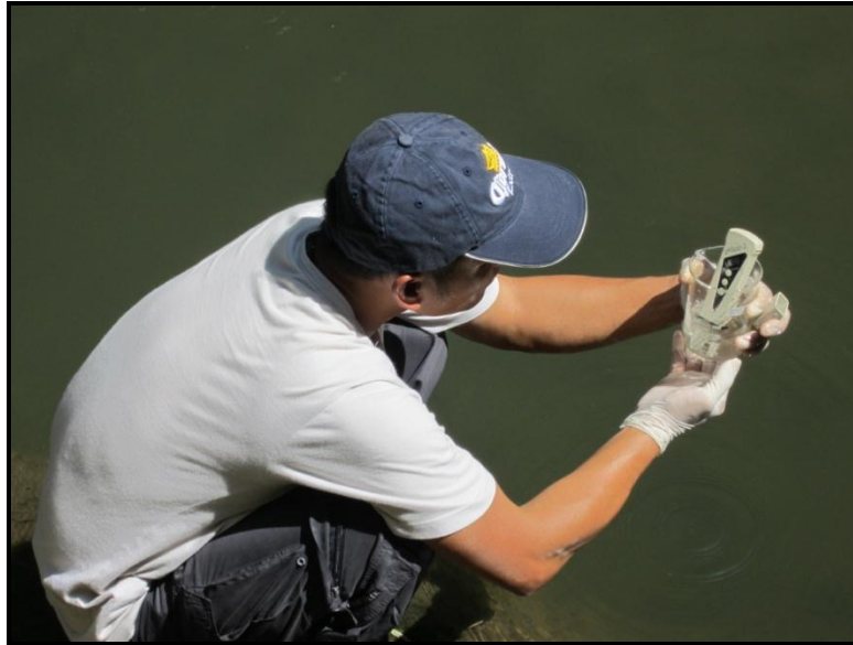
Plate No. 15 On-site pH measurement of the water sample collected from Malaking Ilog River ( Sta. 1 ).
