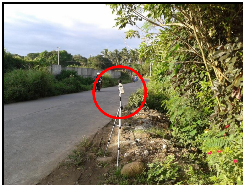
Plate No. 26 Daytime noise level monitoring using a portable Noise Meter at sampling Sta. 3 , Brgy. Tibig, Silang, Cavite.
