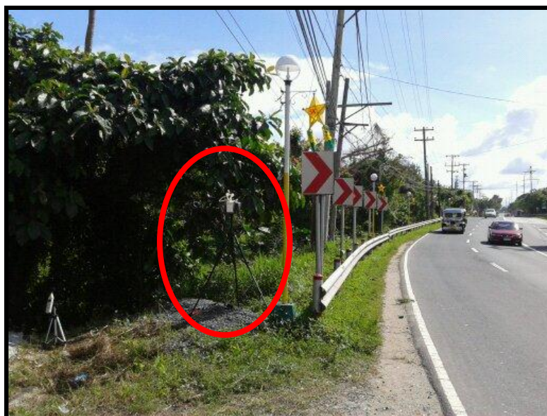
Plate No. 18 Ambient TSP level sampling along E. Aguinaldo Highway, Brgy. Biga II, Silang, Cavite ( Sta. 1 ) using a Staplex High-Volume Sampler (indicated by the red marking).
