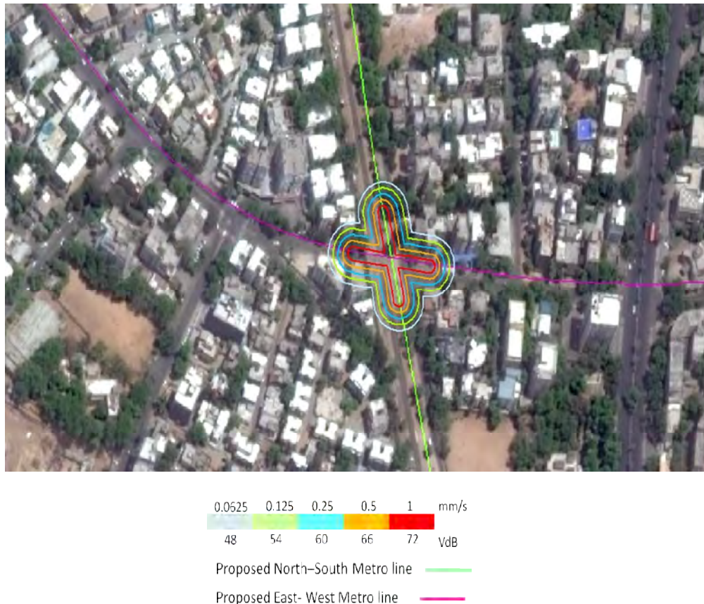
FIGURE 4.15 VIBRATION DUE TO METRO TRAIN AT METRO RAIL CROSSING
