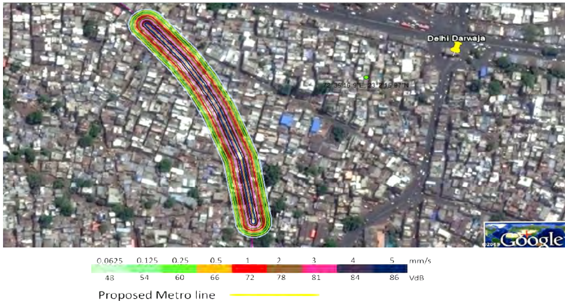
FIGURE 4.2 VIBRATION CONTOURS DUE TO TBM AT DELHI DARWAZA
