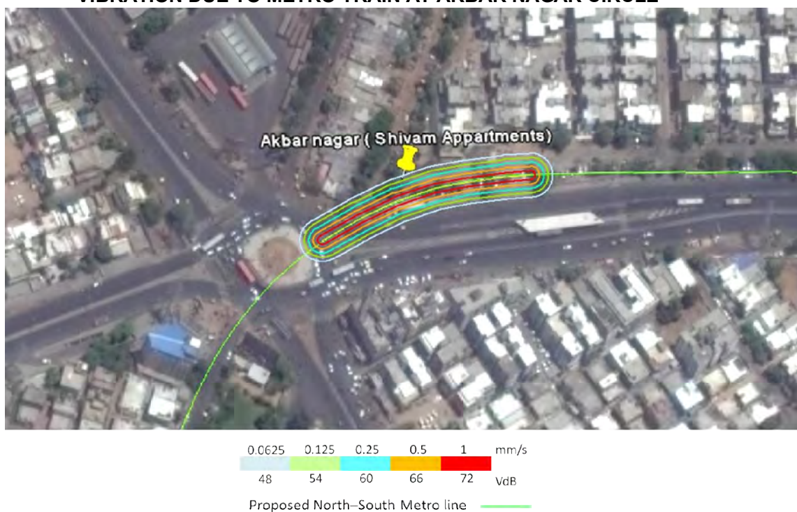
FIGURE 4.17 VIBRATION DUE TO METRO TRAIN AT AKBAR NAGAR CIRCLE
