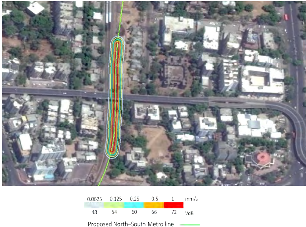
FIGURE 4.16 VIBRATION DUE TO METRO TRAIN AT SILVER ARC APARTMENT
