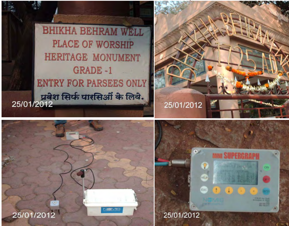
FIGURE 3.45 VIBRATION MONITORING AT LOCATION AT PARSEES WELL, HUTATMA CHOWK
