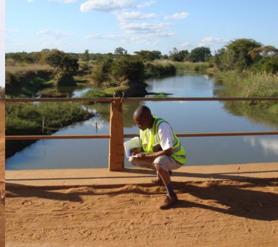
Fig. 2.2 GPS Recording of Bridge Coordinates
