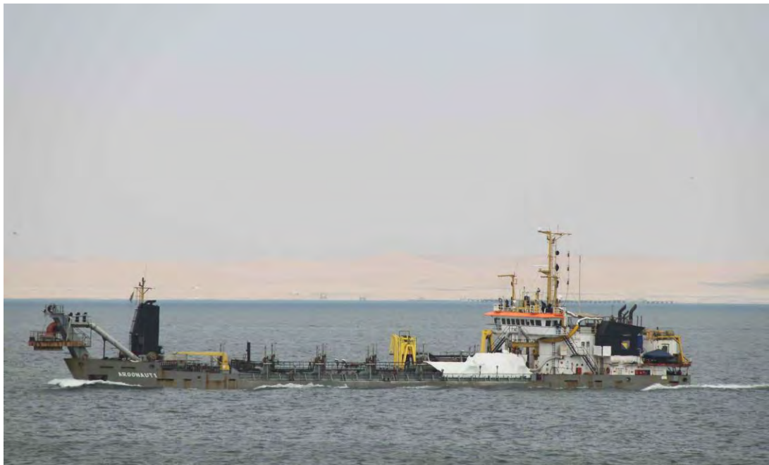
Figure 7.4: Pictorial Illustration of Trailer Suction Hopper Dredger (TSHD) Source: MPDP
