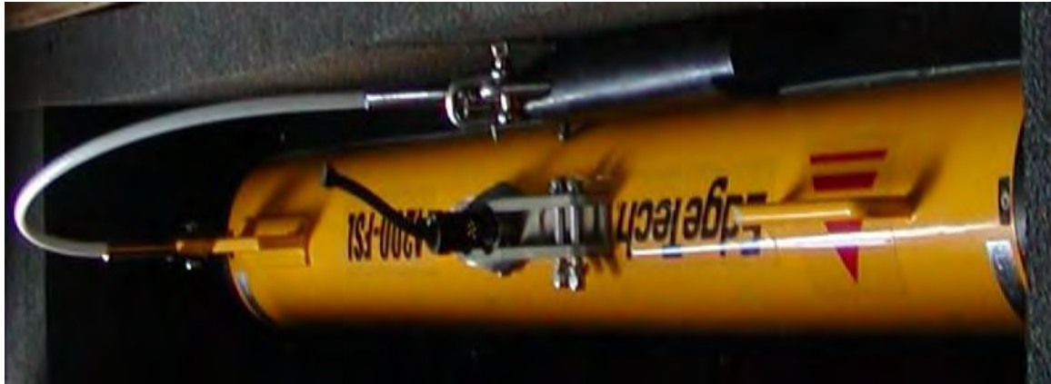
Figure 6.2: Edgetech 701 DL 'Fish' for Side Scan Sonar
