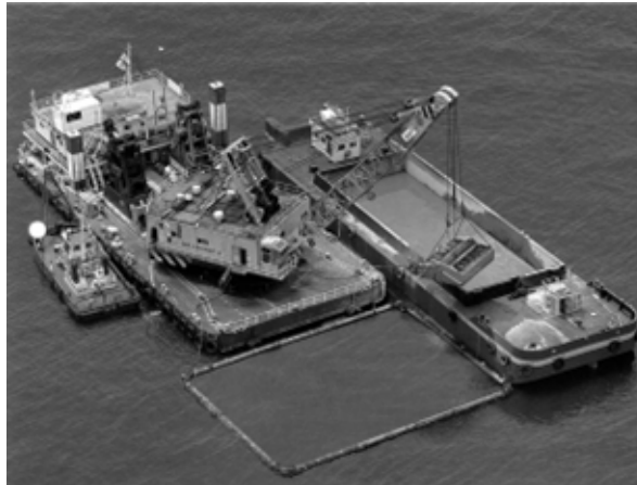
Fig 5.5: Grab Dredge (Contaminated Material Dredging)
